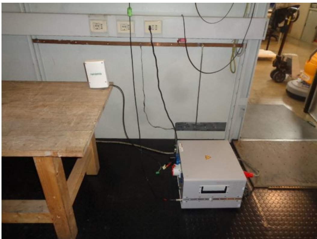
Figure 9.1-3: Conducted emissions set-up
