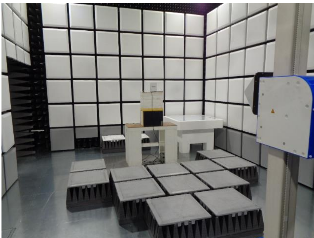
Figure 9.1-2: Radiated emissions set-up for frequencies above 1 GHz
