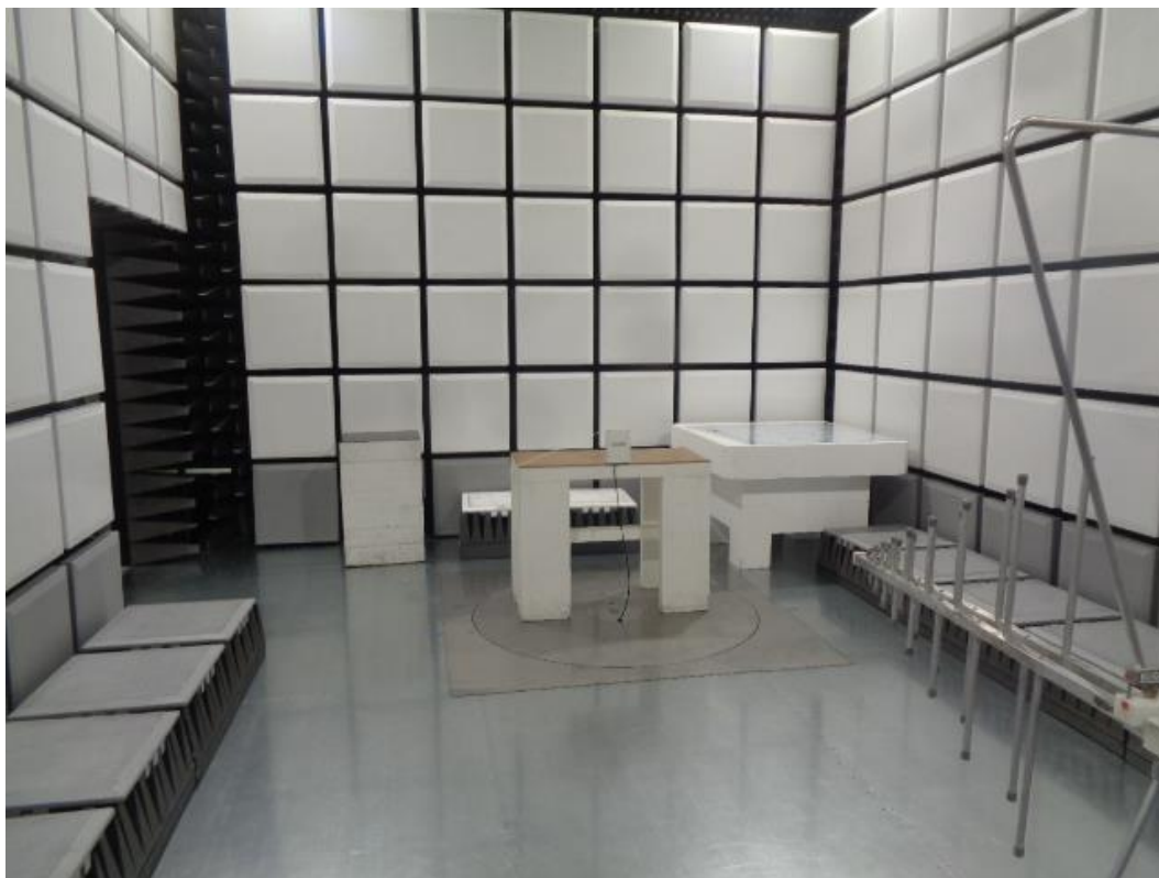
Figure 9.1-1: Radiated emissions set-up for frequencies below 1 GHz
