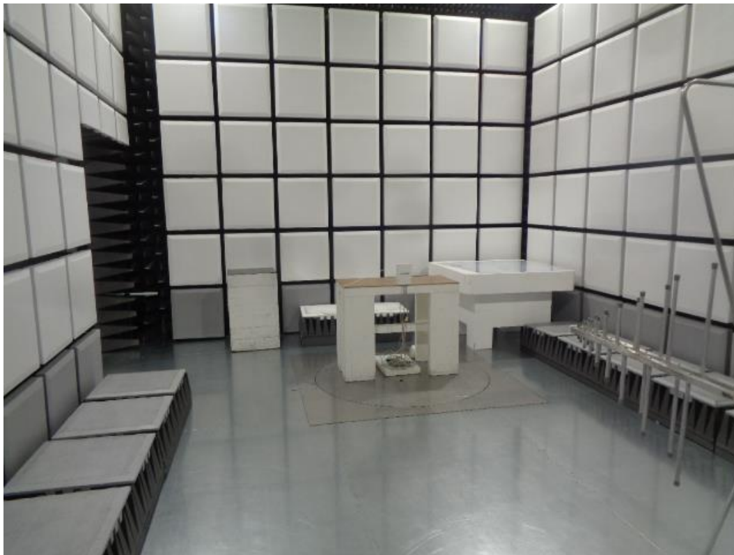
Figure 9.1-1: Radiated emissions set-up for frequencies below 1 GHz
