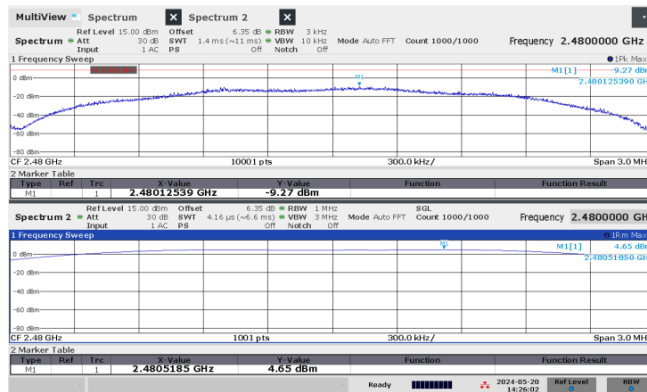
Figure 4.2.4 (i) Power Spectral Density Plots.
