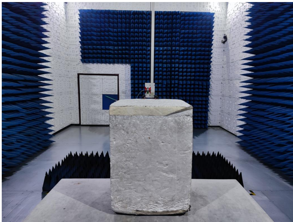
RADIATED EMISSION TEST SETUP ABOVE 1GHz
