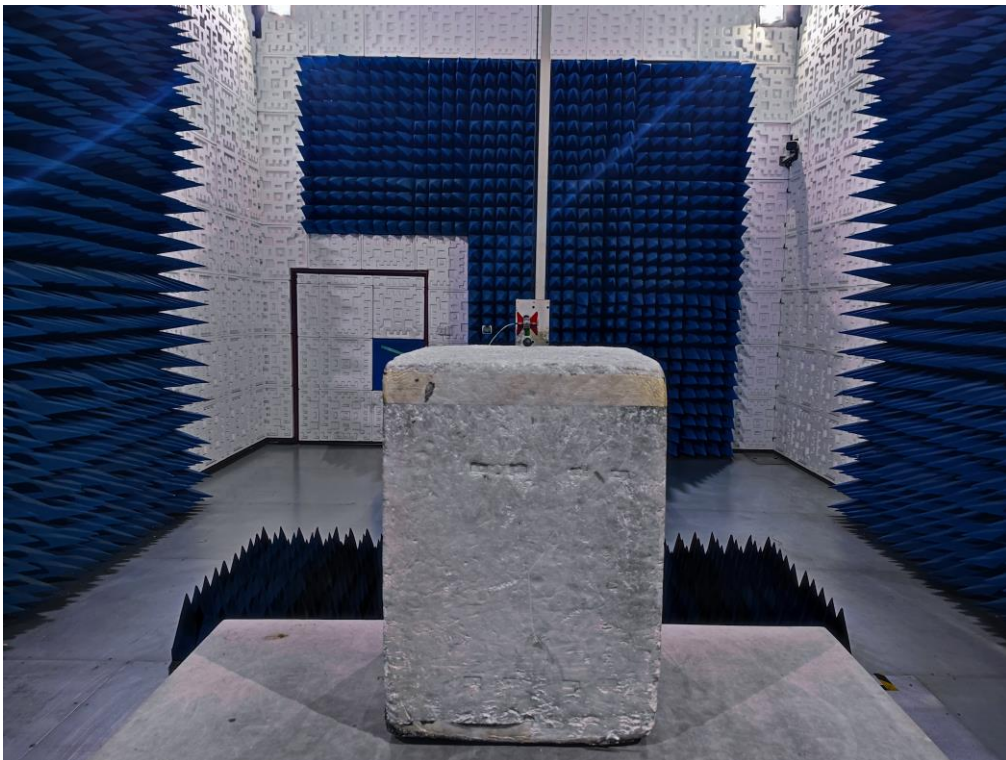
RADIATED EMISSION TEST SETUP ABOVE 1GHZ
