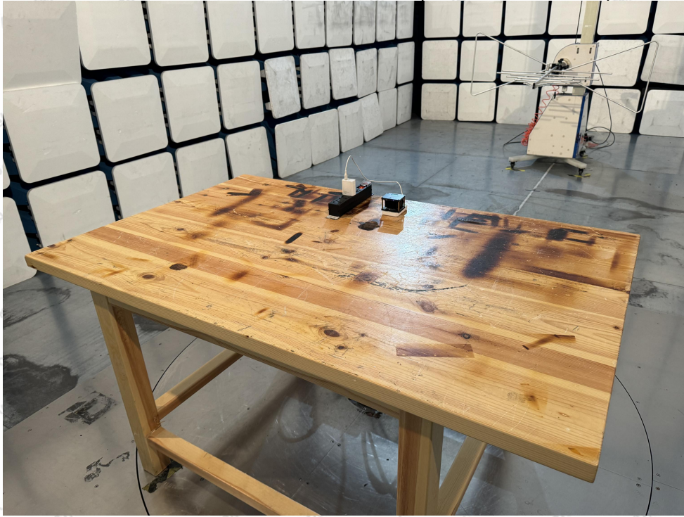
Photo of Radiation Emission Test (30MHz~1000MHz)
