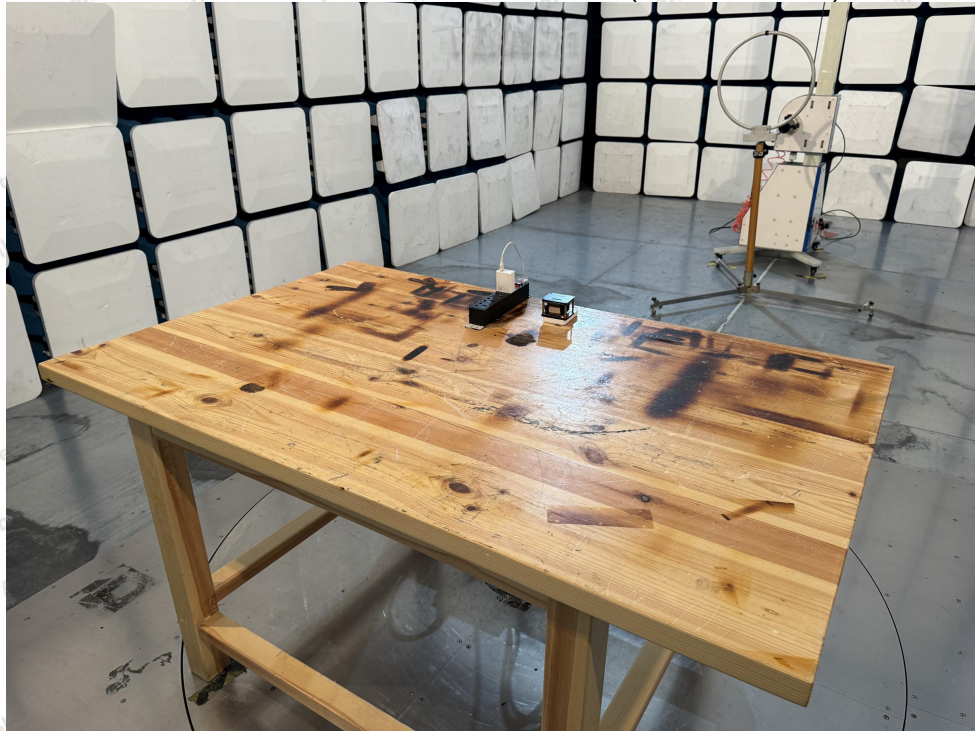
Photo of Radiation Emission Test (below 30MHz)
