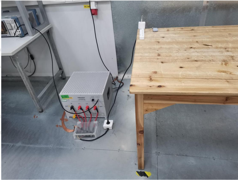
Photo of Conducted Emission Measurement
