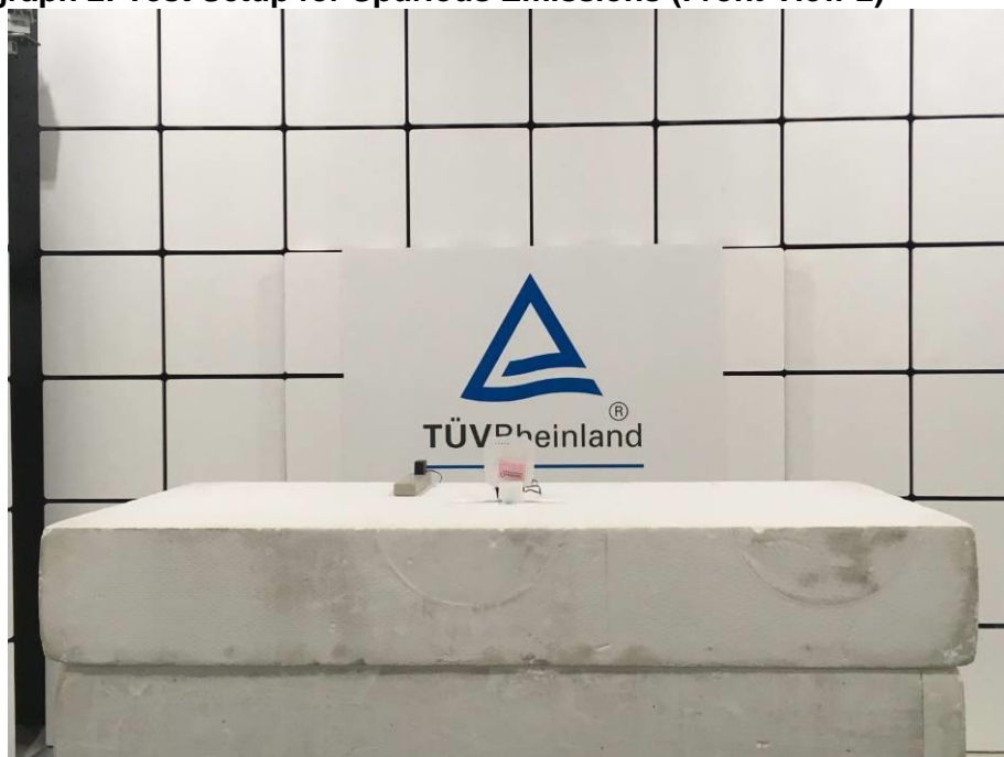
Photograph 2: Test Setup for Spurious Emissions (Front View 2)
