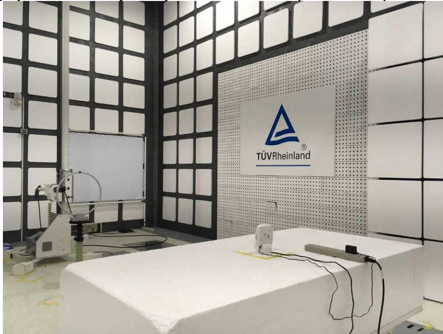
Photograph 4: Test Setup for Spurious Emissions (Back View 2)
