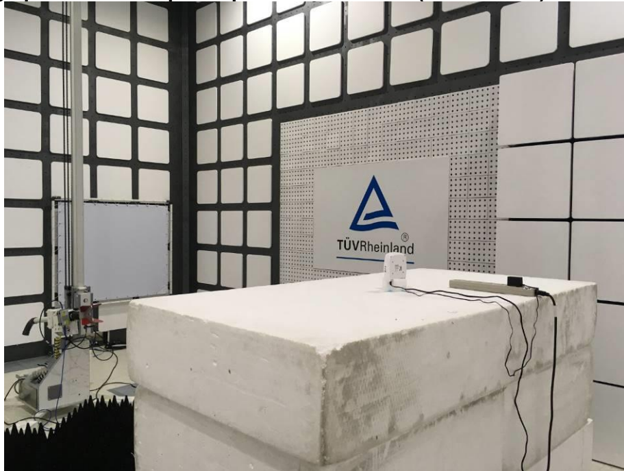
Photograph 6: Test Setup for Spurious Emissions (Back View 4)
