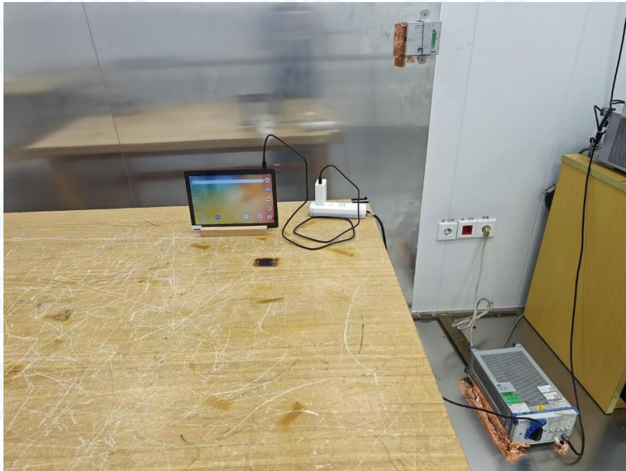
Photo of Setup for Conducted Emission
