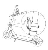
3. Install six screws (two on each side) with the included hex wrench.
