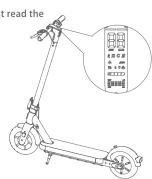
Power on the Scooter and check the power level indicator. Charge the Scooter if the battery level is low.
