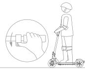
3. Push the scooter forward to reach 2.5 mph (4 km/h), put your other foot on the footrest to keep both feet stable, press the throttle to speed up.
