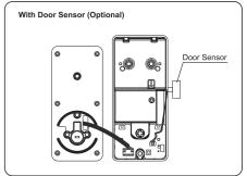
3. Insert the front body cable through the rectangular hole the rubber pad. Connect the wire connector from the front body through the hole to the back body. Ensure that the wire is installed properly and securely.
