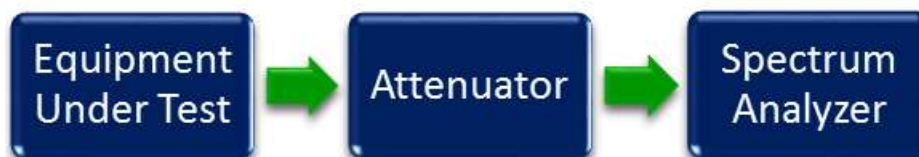
Figure 3. Occupied Bandwidth Test Setup
