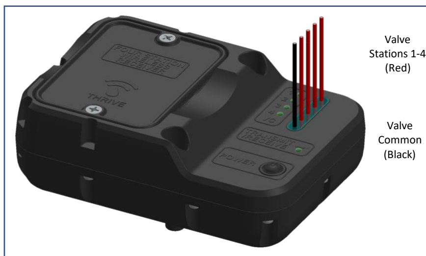
Field Wire Connections to Receiver™ Figure 11-1
