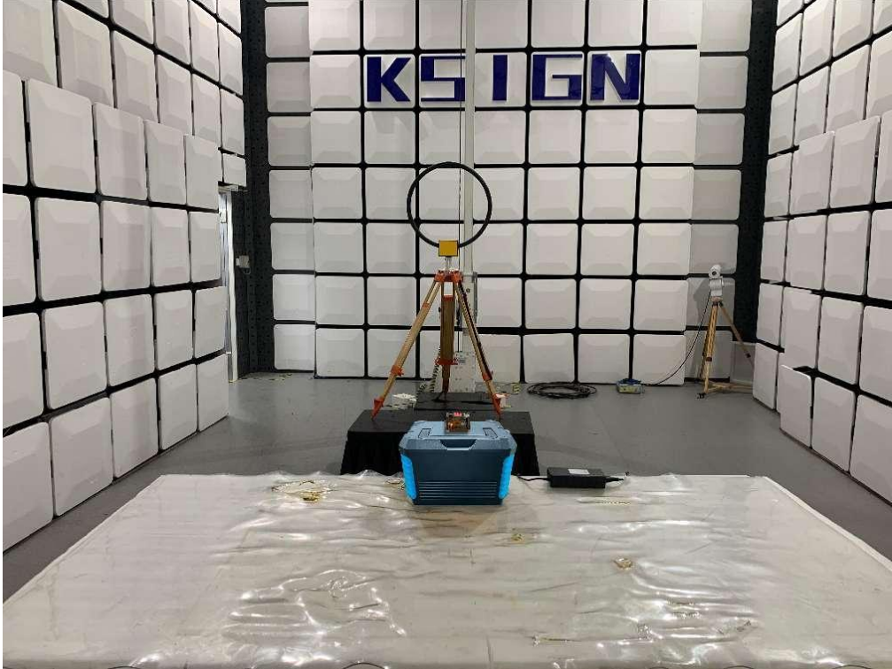
Radiated Measurement (Below 30MHz)
