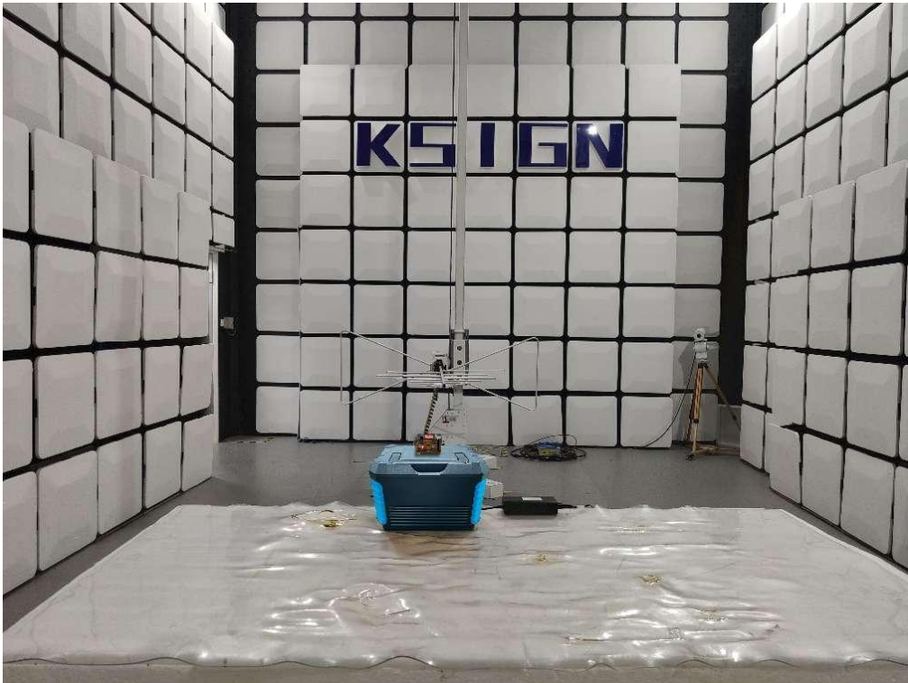
Radiated Measurement (Above 30MHz)
