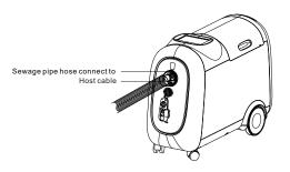
$\ensuremath{\textcircled{2}}$  Turn the hose connector clockwise to lock in the Host connection section
