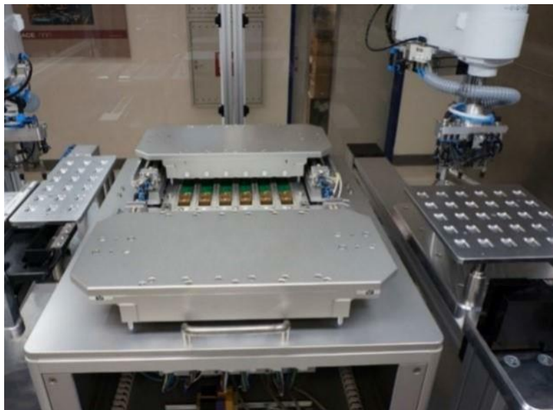
Figure 10: Automatic test equipment for module test
