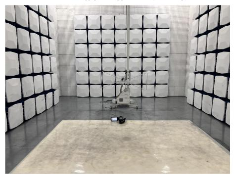
RADIATED EMISSION MEASUREMENT (Above 1G)
