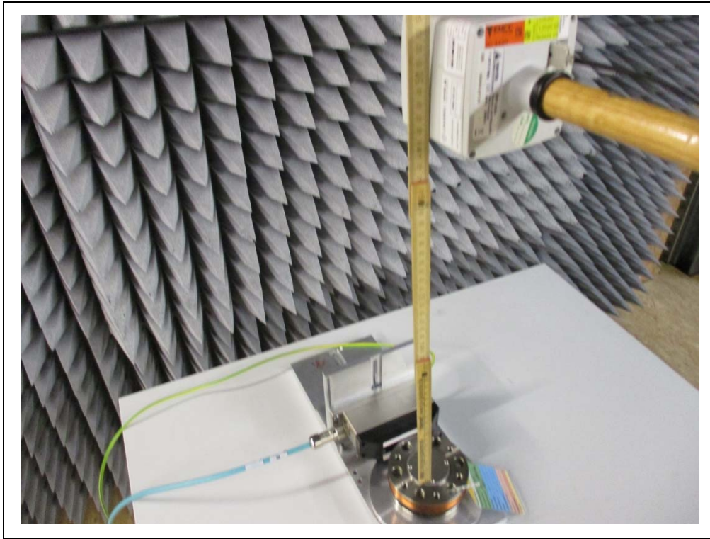
Photograph 4.1 - 1: EUT DF1 plus Distance EUT to field probe 50 cm (Setup A)
