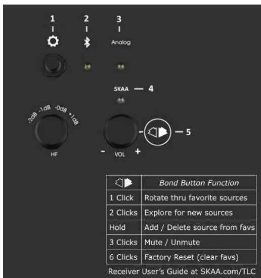
Figure 2: SKAA Bond Button & Bonding Table
