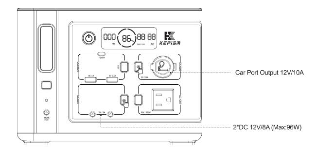
Note: DC5521, single-port maximum load capacity is 12V\*8A, dual-port simultaneous workload capacity of dual-port parallel is maximum 12V\*8A. The port will be protected automatically when overloaded. The output can be restored automatically after disconnecting the load. Press and hold the DC5521 button for 1 second to turn off the output of this port.
