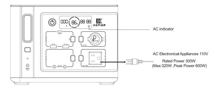
The AC output of this product has 2 functional modes: energy saving mode and online mode. A:energy-saving mode: After turning on the AC output switch, the AC port will shut down automatically if no electrical appliance is plugged in within 1 minute, or the power of the electrical appliance is less than 10W.
