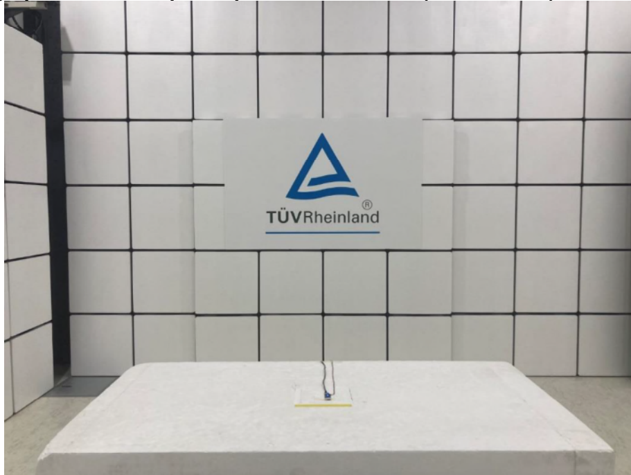
Photograph 2: Test Setup for Spurious Emissions (Front View 2)
