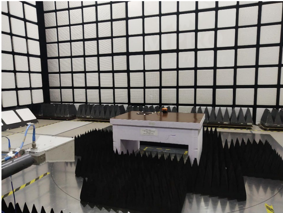
Figure 9: Photograph of RE test setup from 1 GHz to 18 GHz_ Vertical polarization
