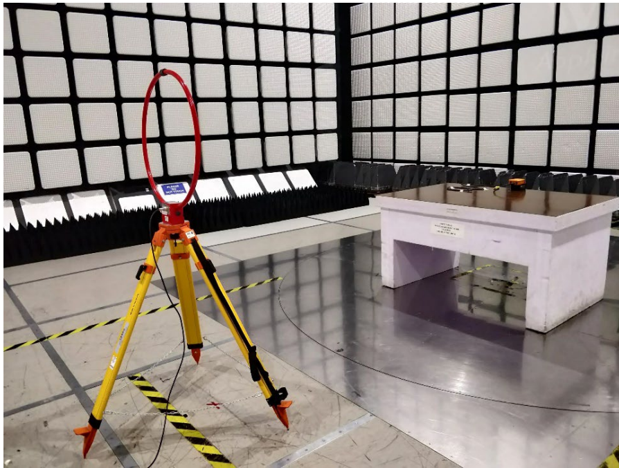
Figure 1: Photograph of RE test setup from 9 kHz to 30 MHz _ Parallel to EUT
