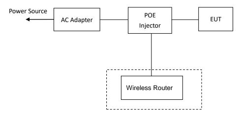
Note: for reference only, the actual connection setup used for testing please refer to the test photos.
