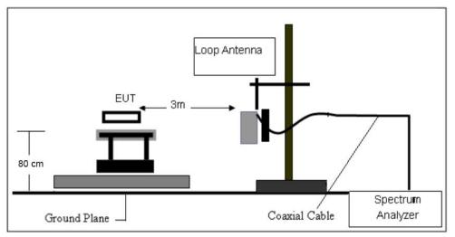
(B) Radiated Emission Test-Up Frequency 30MHz~1GHz
