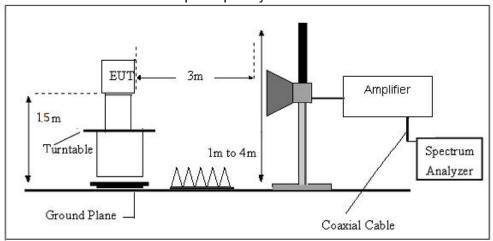
Radiated Emission Test-Up Frequency Above 1GHz
