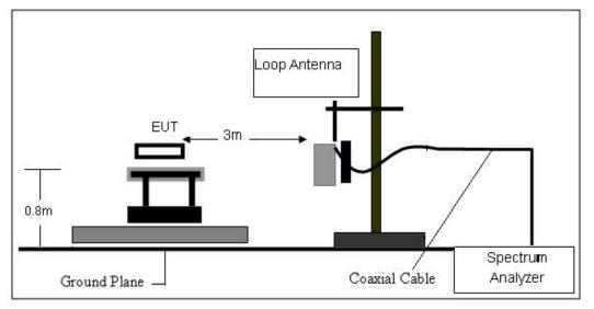
(B) Radiated Emission Test-Up Frequency 30MHz~1GHz
