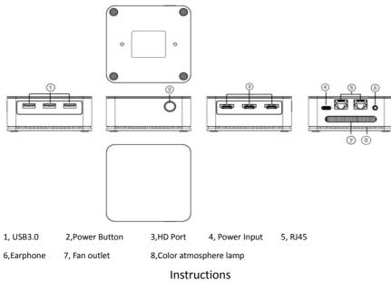
1. Connect the device with the display device (such as TV, screen, projector, etc.) via HD line, and select the "video input source" of the display device to the connected HD input channel.
