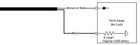
\*Note: Care must be taken when selecting Loop resistor. The RADAR needs a minimum of 12V to operate. If Loop resistor is to large it will starve the RADAR unit and erroneous output may occur.
