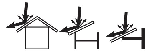
Install the sensor as perpendicular as possible to the media surface to obtain the most accurate measurement readings. The middle of the sensor face is the beginning of the measurement range.
