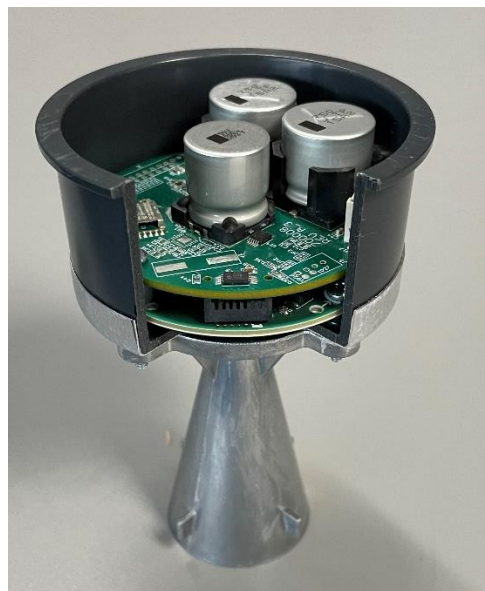
Picture 2- Cut away view of Cup and Horn assembly.
