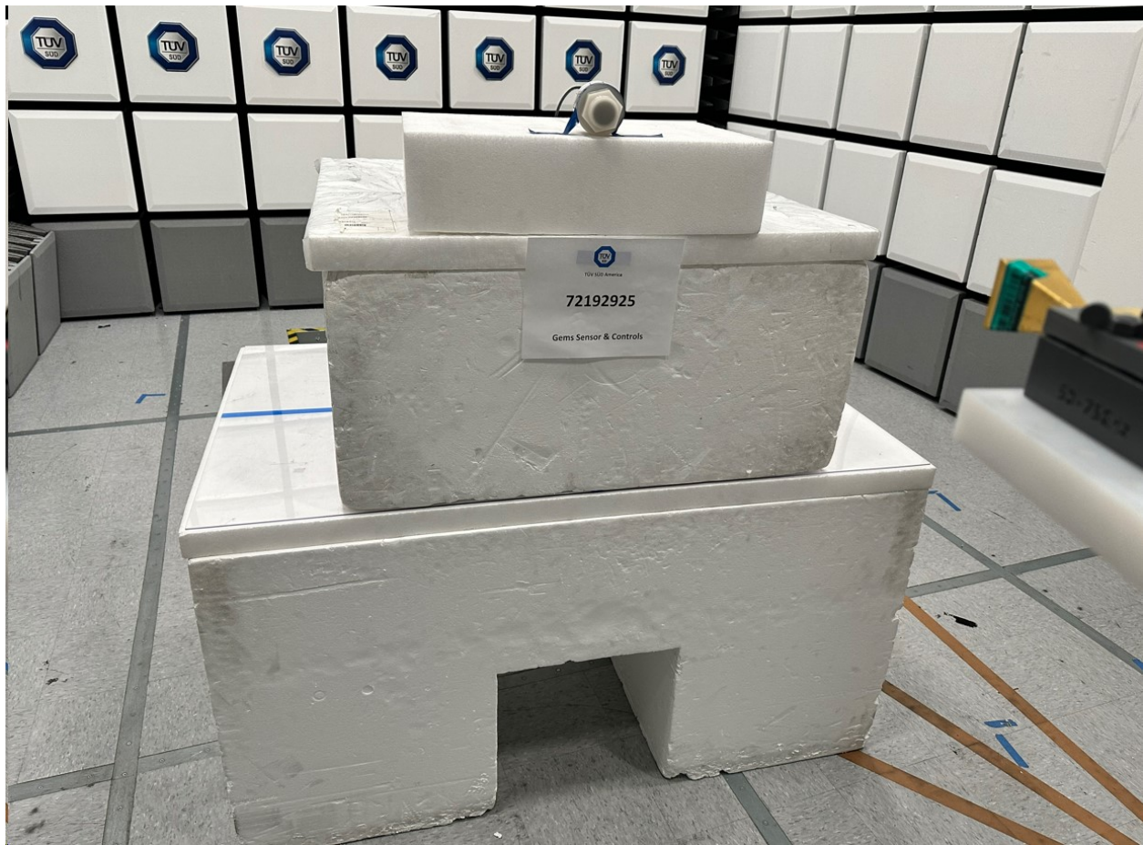
Radiated Emissions Test Setup (60GHz to 75GHz)
