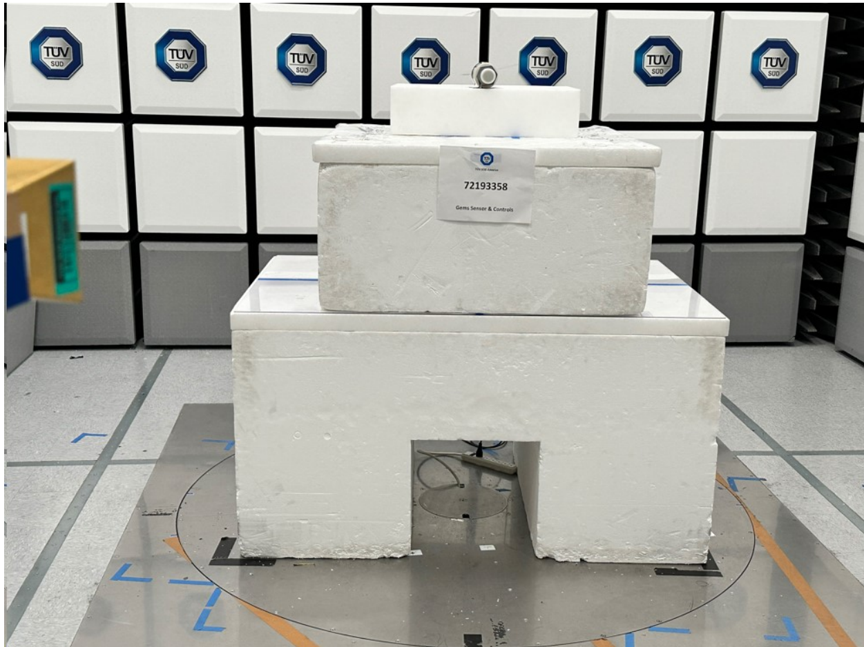
Radiated Emissions Test Setup (26GHz to 40GHz)
