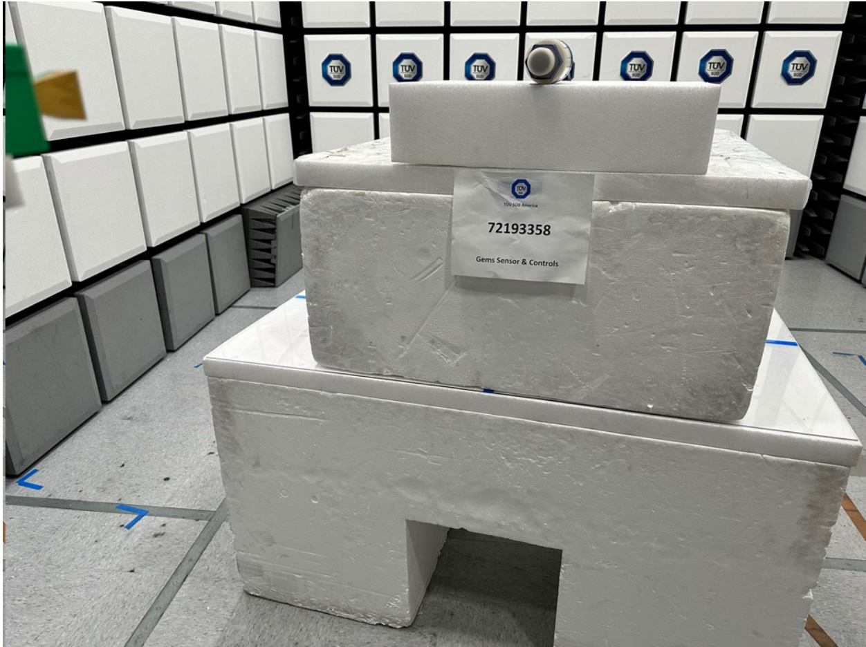
Radiated Emissions Test Setup (75GHz to 110GHz)
