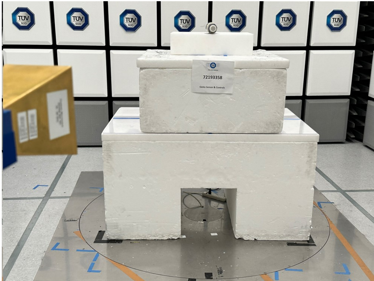
Radiated Emissions Test Setup (18GHz to 26GHz)
