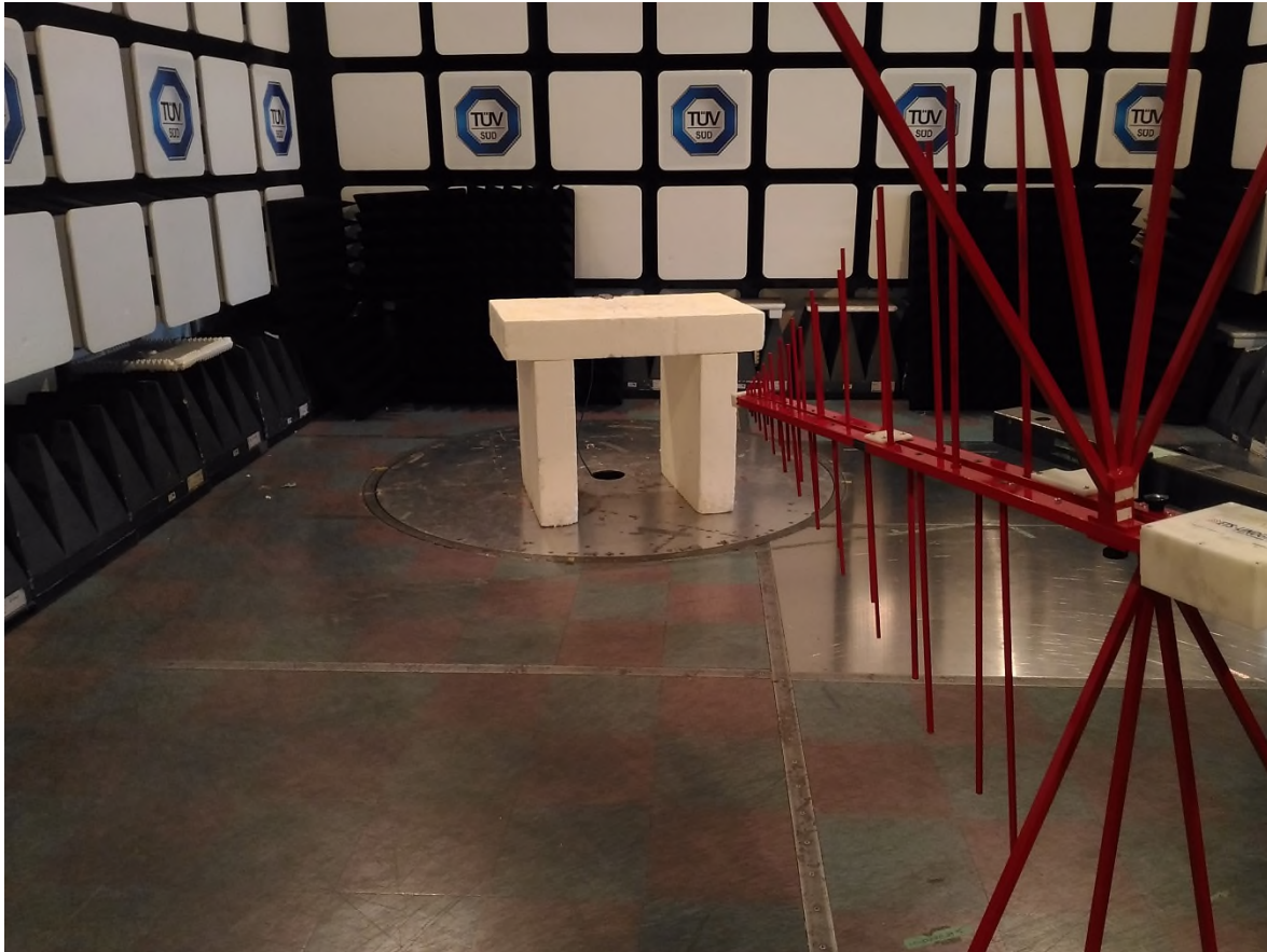
Figure 3 – Radiated Emissions Setup 30 MHz to 1 GHz
