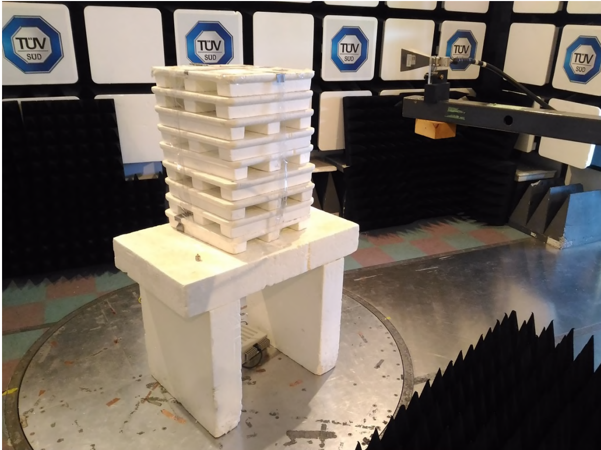
Figure 6 – Radiated Emissions Setup 18 GHz to 25 GHz
