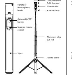
First of all, pull the handle of the mobile phone holder out along upward direction and drop it vertically from a height of about 10cm from the ground; then the tripod of selfie stick will bounce automatically.
