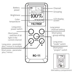
1.Long press RC-11 "power switch" for 2 seconds, waiting for the power turning on and the display screen being on.
