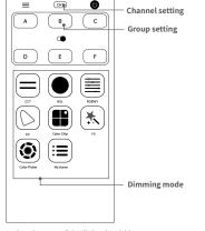
The channel and group of the light should be consistent with the mobile bluetooth APP.
