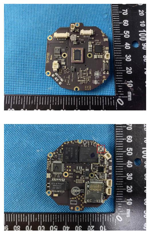
Inside the red square is the soldering point of the coaxial cable between the antenna connector and the mainboard.
