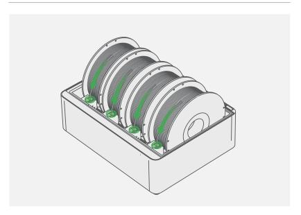
Place at least one spool of Bambu Filament into the AMS. Turn on the power to start the printer and the AMS. Insert the filament into the filament inlet. The filament will be automatically pre-loaded when detected.
