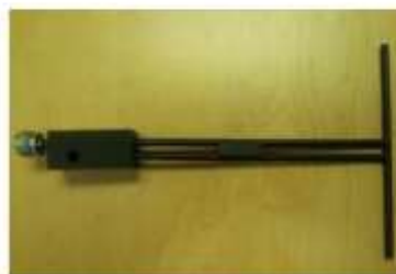
Figure 1 – MVG COMOSAR Validation Dipole
