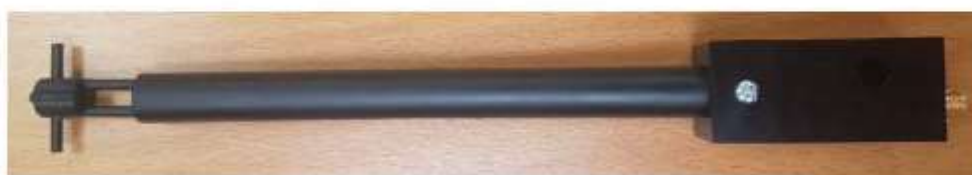
Figure 1 – MVG COMOSAR Validation Dipole
