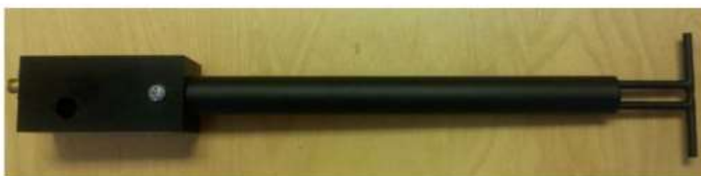
Figure 1 – MVG COMOSAR Validation Dipole
