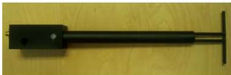
Figure 1 – MVG COMOSAR Validation Dipole
