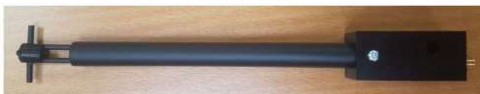
Figure 1 – MVG COMOSAR Validation Dipole
