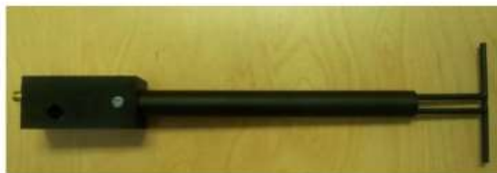
Figure 1 – MVG COMOSAR Validation Dipole
