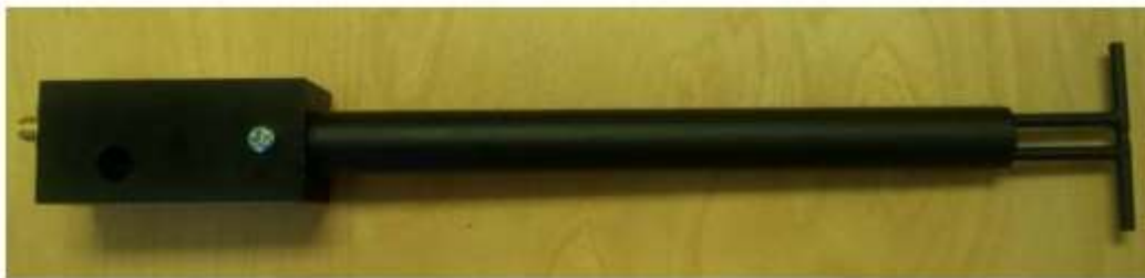
Figure 1 – MVG COMOSAR Validation Dipole
