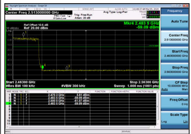
Conducted Emission: 8DPSK,2480,3DH5 ,Band Edge
