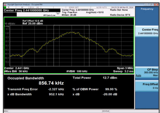
20dB Bandwidth: DQPSK,2402MHz,2DH5
