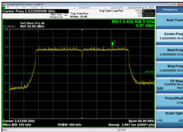
,Plot 1,Reference Level-802.11ax(40MHz),2437MHz,Ant13
