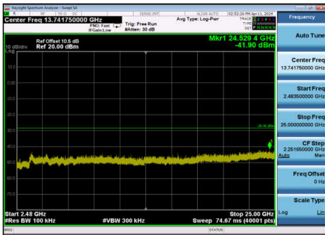
,Plot 4,2483.5MHz~25000MHz-802.11n(40 MHz),2437MHz,Ant13
