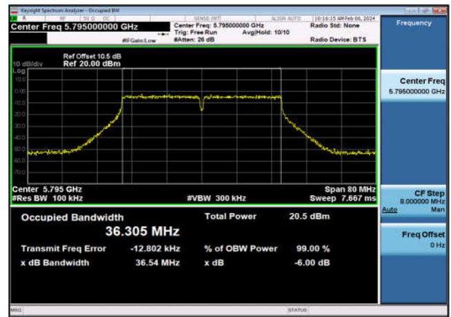
U-NII-3 6dB Bandwidth-802.11ac(80MHz) ,5775MHz,Ant11
