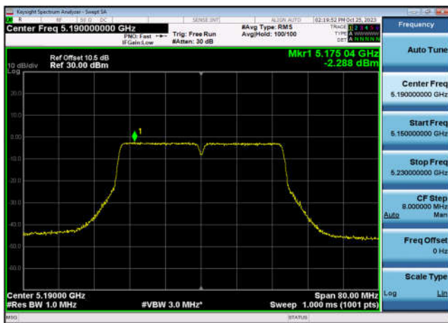
U-NII-1 Power spectral density-802.11 ac(40MHz),5190MHz,Ant9
