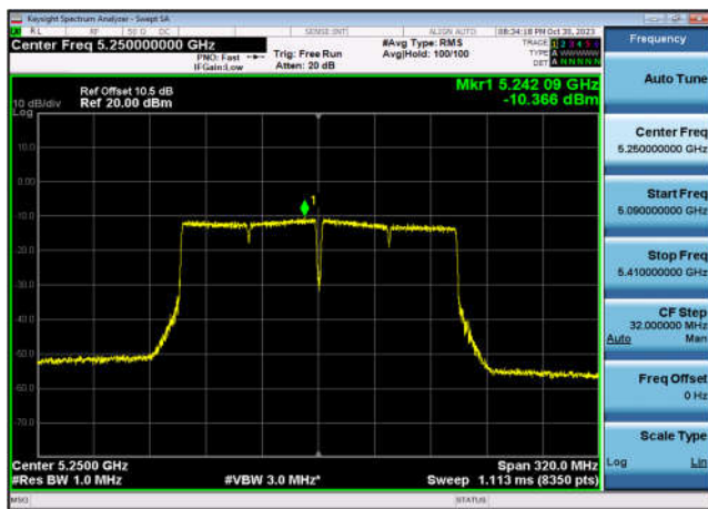
U-NII-2a Power spectral density-802.1 1ac(20MHz),5260MHz,Ant9
