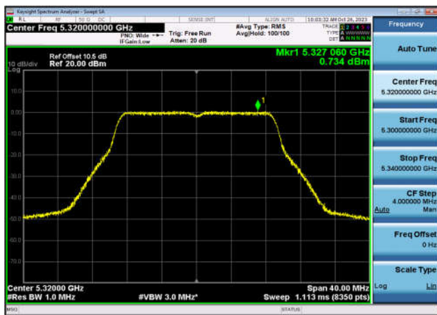
U-NII-2a Power spectral density-802.1 1n(40MHz),5270MHz,Ant9
