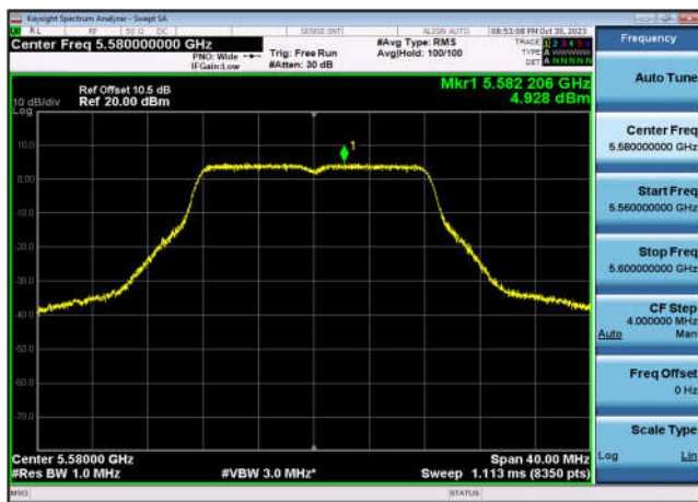
U-NII-2c Power spectral density-802.1 1a(20MHz),5700MHz,Ant9
