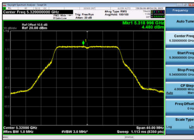
U-NII-2a Power spectral density-802.1 1ac(160MHz),5250MHz,Ant9
