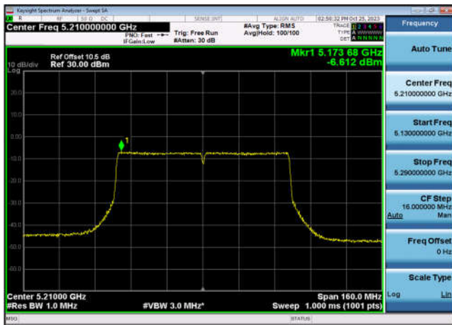
U-NII-1 Power spectral density-802.11 ax(20MHz),5180MHz,Ant9
