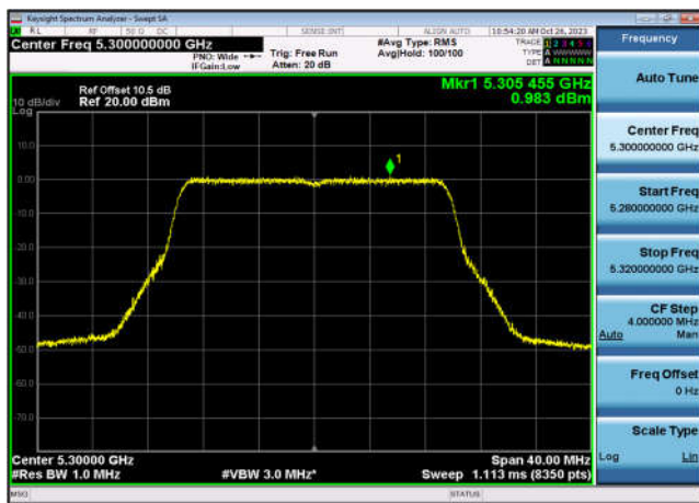
U-NII-2a Power spectral density-802.1 1ax(20MHz),5320MHz,Ant9
