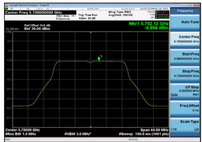
U-NII-2c Power spectral density-802.1 1ac(40MHz),5510MHz,Ant10
