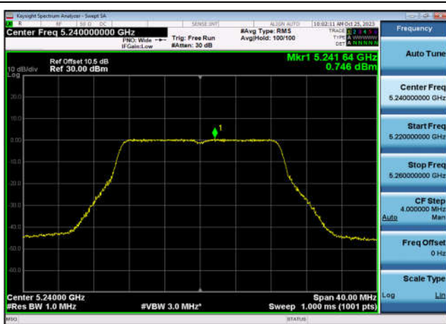
U-NII-1 Power spectral density-802.11 n(20MHz),5240MHz,Ant9
