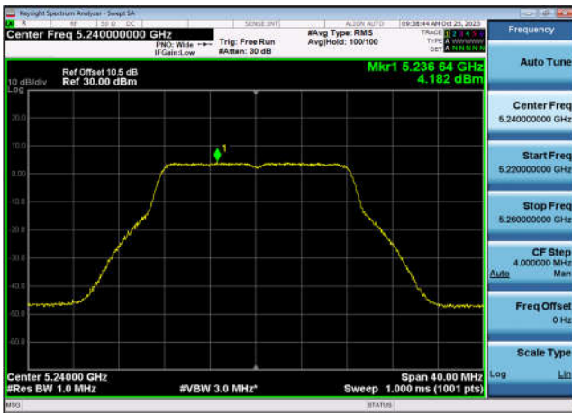
U-NII-1 Power spectral density-802.11 ac(20MHz),5180MHz,Ant9
