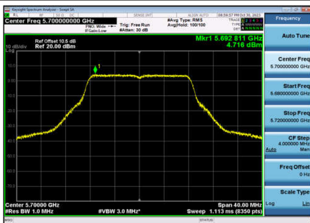
U-NII-2c Power spectral density-802.1 1a(20MHz),5700MHz,Ant9
