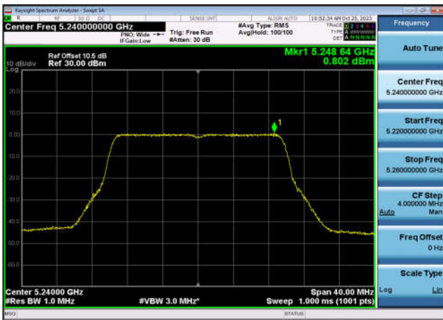
U-NII-1 Power spectral density-802.11 ax(40MHz),5190MHz,Ant9
