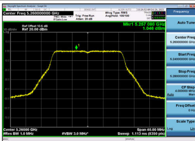
U-NII-2a Power spectral density-802.1 1ac(20MHz),5260MHz,Ant9
