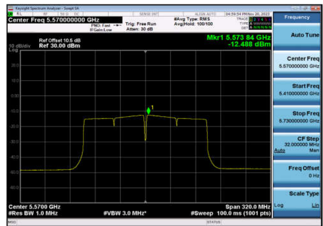
U-NII-2c Power spectral density-802.1 1ac(20MHz),5500MHz,Ant10
