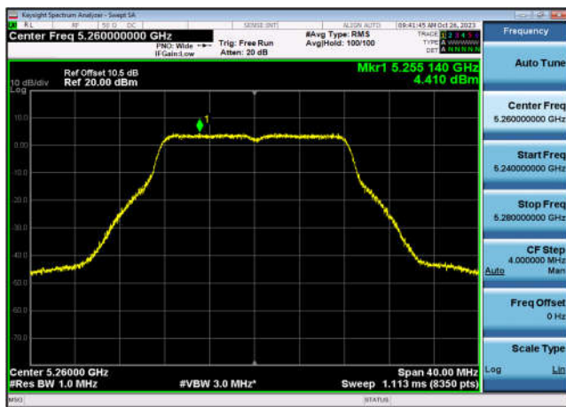
U-NII-2a Power spectral density-802.1 1a(20MHz),5300MHz,Ant9
