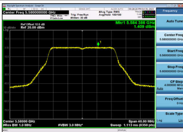
U-NII-2c Power spectral density-802.1 1ac(20MHz),5580MHz,Ant9
