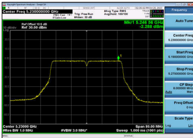
U-NII-1 Power spectral density-802.11 a(20MHz),5180MHz,Ant9
