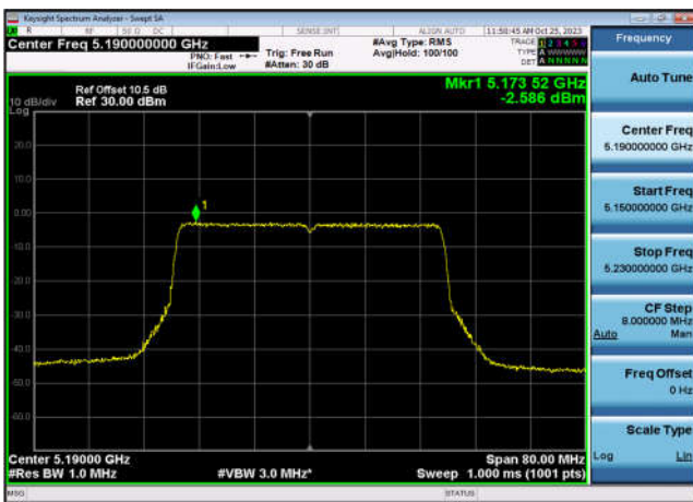
U-NII-1 Power spectral density-802.11 ax(40MHz),5190MHz,Ant9
