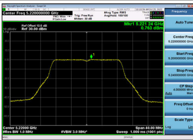
U-NII-1 Power spectral density-802.11 n(20MHz),5240MHz,Ant9
