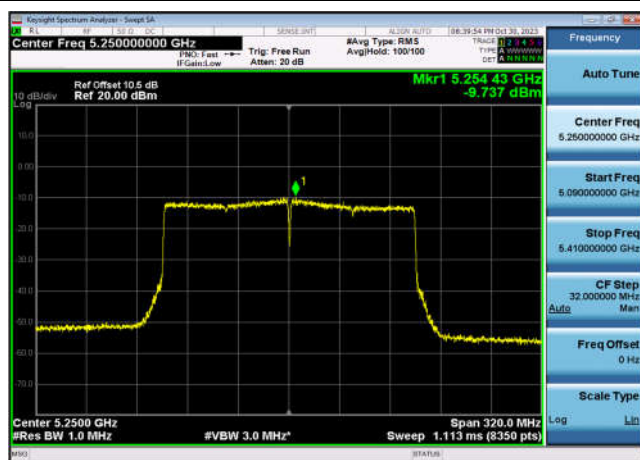
U-NII-2a Power spectral density-802.1 1ax(160MHz),5250MHz,Ant9
