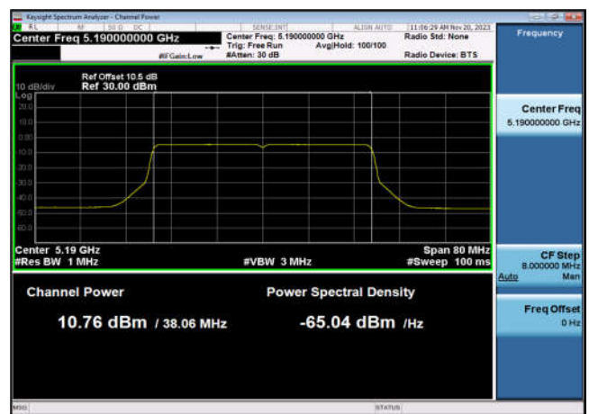
U-NII-1 Output Power-802.11ax(40MHz) ,5190MHz,Ant10
