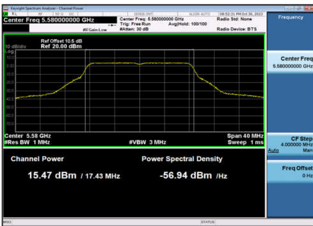
U-NII-2c Output Power-802.11a(20MHz) ,5700MHz,Ant9
