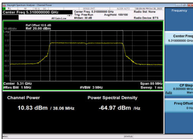
U-NII-2a Output Power-802.11ax(80MHz) ,5290MHz,Ant9
