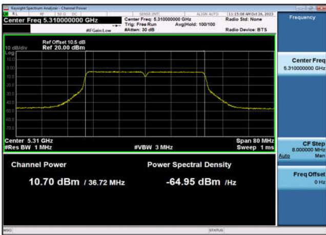
U-NII-2a Output Power-802.11a(20MHz) ,5260MHz,Ant9
