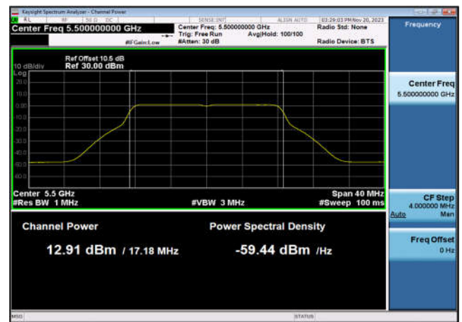
U-NII-2c Output Power-802.11a(20MHz) ,5580MHz,Ant10
