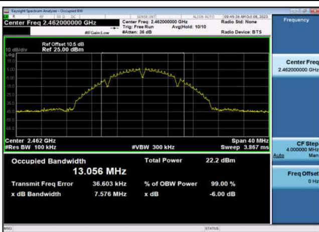
6dB Bandwidth-802.11b,2462MHz,Ant7
