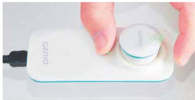
Figure 13: Blinking Activation Chip LED upon connection to the Charging Unit, indicating charging.
