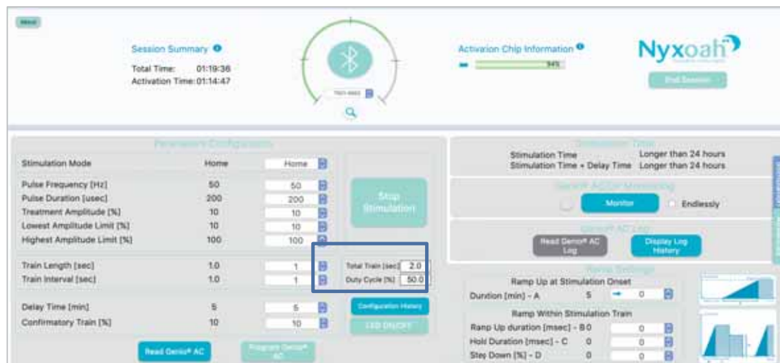
Figure 46: AC Parameters automatically calculated by the Genio® Patient Application, Total train length and Duty Cycle
