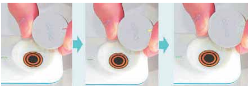
Figure 17: Red/Yellow/Green LED Indications on the Activation Chip following reset in the Charging Unit
