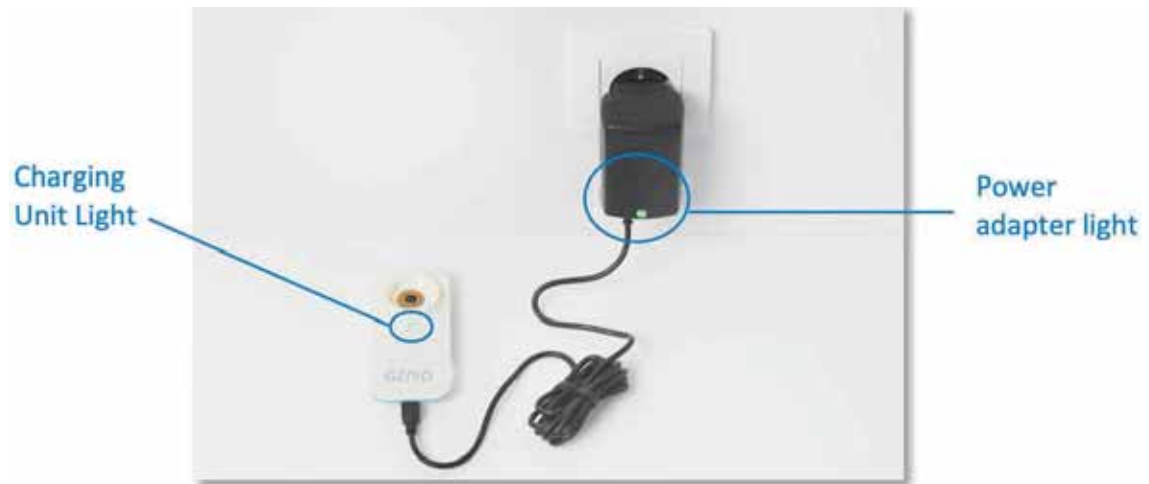
Figure 11: Charging Unit and power adapter light upon connection to power
