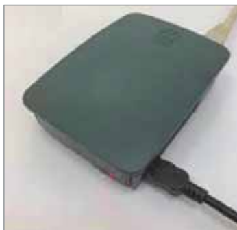
Figure 16: Repeater connected to Ethernet cable and power cable
