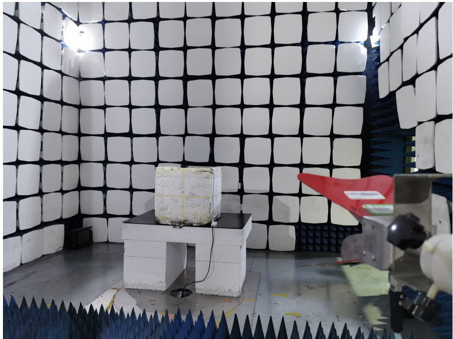
Radiation Emission Test Setup (1GHz to 18GHz)
