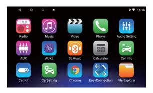
With your finger in the upper right area of the main interface to decline, you can quickly open the Settings/ Car Settings/ Memory Clean/WLAN Closed/ Luminance/ Sound function setting interface.
