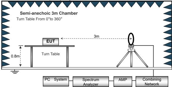
(B) Radiated Emission Test-Up Frequency 30MHz~1GHz
