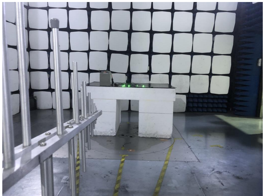
Radiation Emission Test Setup (30MHz to 1GHz)
