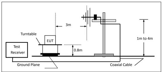
(c) For radiated emissions above 1000MHz
