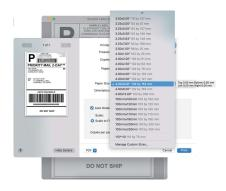
3.Select "Printer Features", then change the settings of printer, e.g Speed, Darkness, Rotate.
