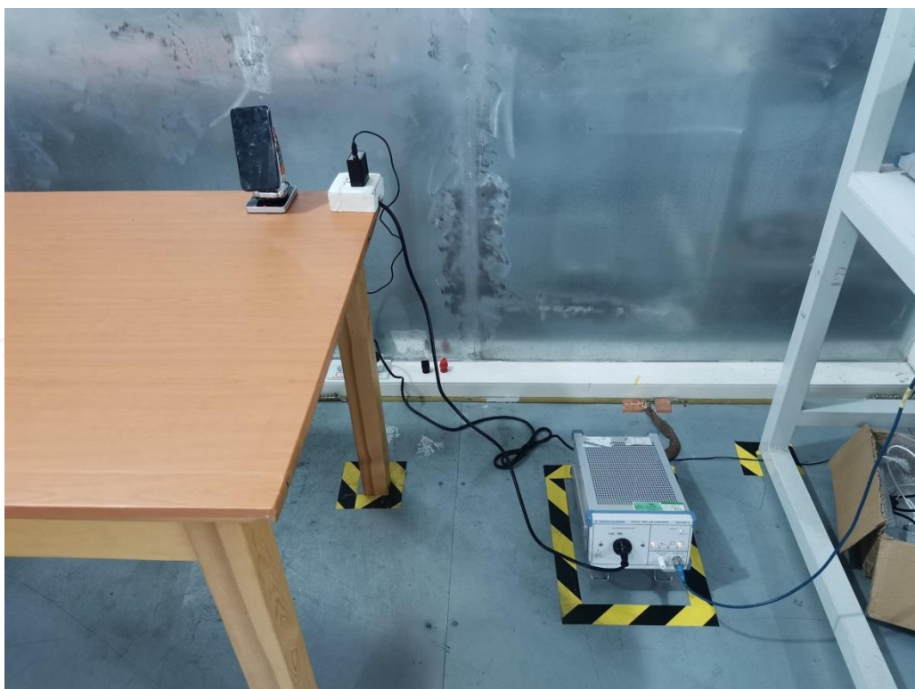
Conducted Emission-AC adapter charge mode
