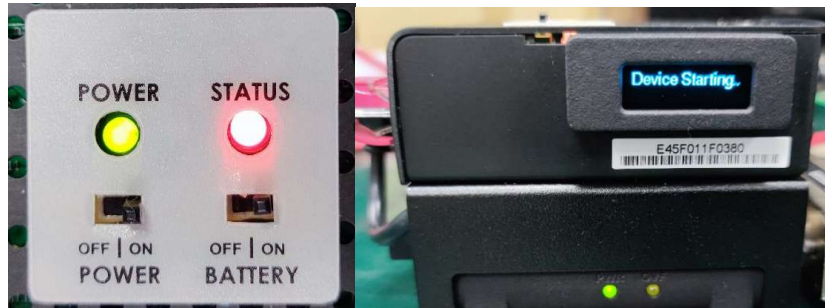
Figure 6: GCube4.0 Status LED and display status
