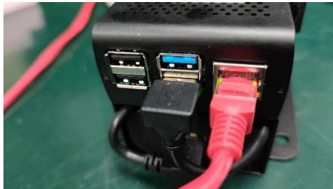
Figure 4: LAN cable connection to GCube4.0
